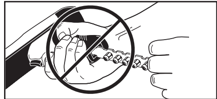
NEVER LOAD THE TOOL UNLESS IT IS TO BE USED IMMEDIATELY
