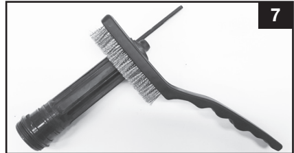
USE BRUSH TO CLEAN OUTSIDE BARREL
