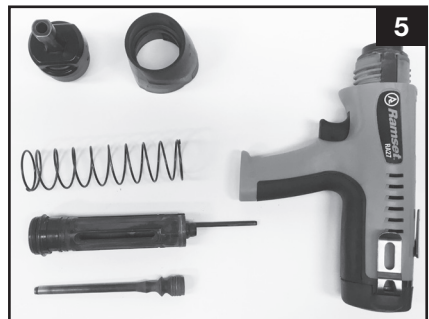
REMOVE THE RETURN SPRING
