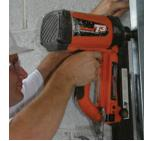
The T3 has enough power to fasten into hard concrete and steel and still will not blow through hollow block.
