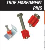
The Ramset .157 True Embedment Pin is sized to provide you with True Embedment depths in track up to 14 gauge. Sized a 1/16" longer than nominal length to provide a True Embedment. 100 per box.
