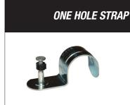
Used to attach EMT conduit or armored cable to concrete. Fastener pre-assembled to a 16 gage conduit strap. 100 per jar, 3/8" 200 per jar.
