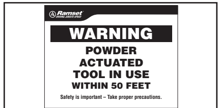
ALWAYS POST WARNING SIGNS
