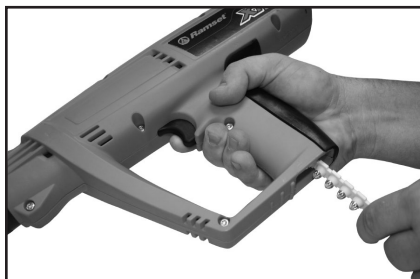
2. INSERT THE POWER LOAD
