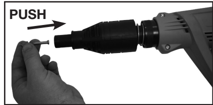
1. SELECT AND INSERT THE FASTENER
