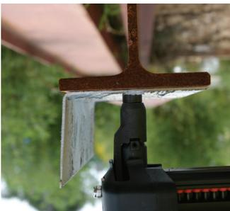
The T3 has enough power to fasten into hard concrete and steel and still will not blow through hollow block.
