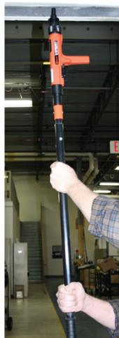
The VIPER4 screws solidly onto a pole for high reach and secure operation for ceiling applications.
