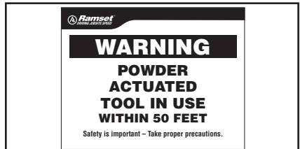
ALWAYS POST WARNING SIGNS
