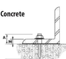
$$\text{Thread Length (A)} = \text{Thickness of Material (M)} + \text{Allowance for Nut \& Washer}^*$$
