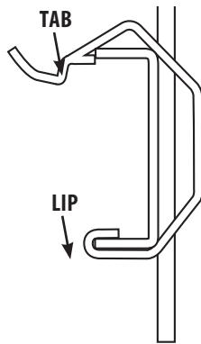
1. Compress the clip and position on the rod at the desired location.
