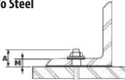
$$\text{Thread Length (A)} = \text{Thickness of Material (M)} + \text{Allowance for Nut \& Washer}^*$$
