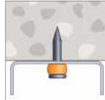
Settling aggregate is the biggest reason for overhead pin failure.
