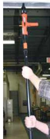
The VIPER4 screws solidly onto a pole for high reach and secure operation for ceiling applications.
