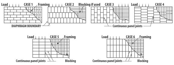
Note: Framing is permitted to be oriented in either direction for diaphragms, provided sheathing is designed for vertical loading.
