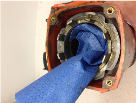
4. After removing much of the dirt, debris, oil, etc. with the spray cleaner, a disposable cleaning wipe can be used to further remove stubborn debris. The end of a hammer handle in conjunction with the wipe can be used to remove debris at the bottom of the cylinder bore.
