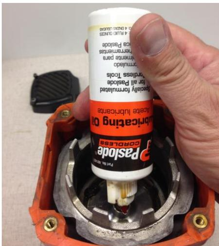
12. Oil is also used to lubricate the walls of the cylinder in the motor assembly. Push the piston down, apply several drops of oil around the walls of the cylinder. Move the piston up and down to help distribute the oil. Also add several drops of oil to the sealing area between the bottom of the combustion chamber and top of the cylinder or sleeve.
