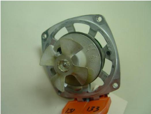
7. Inspect the fan blade and o-ring or steel rings. The fan blade must not be damaged or bent. The o-ring or steel rings must move freely within their grooves.
