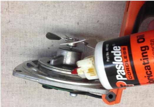
11. Oil is placed onto the steel rings or o-ring area of the cylinder head. Free rotational movement of the ring(s) is desired.
