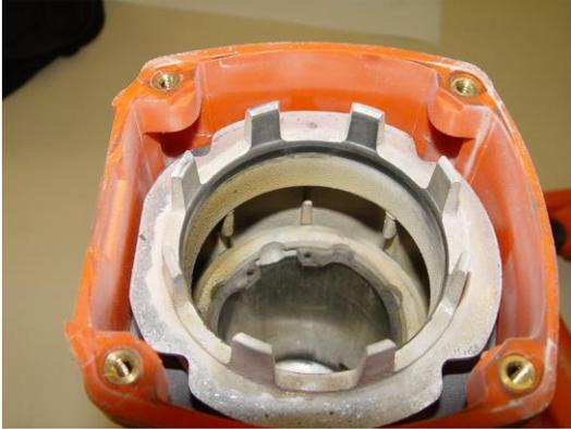
1. Pictured to the left are two examples of a dirty T3 motor housing assembly. There are several very different kinds of dirt.
