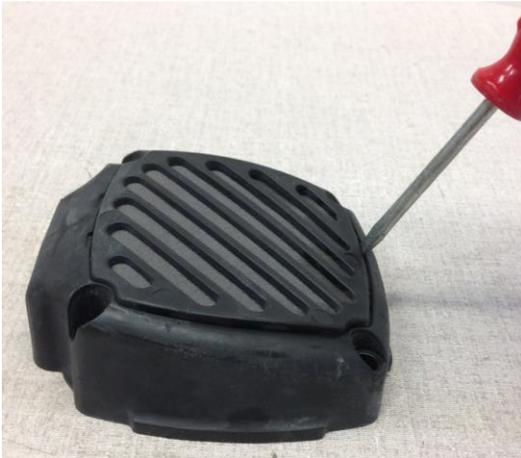
14. Locate the cap and grill assembly. With a flat blade screw driver pry the grill free from the cap.
