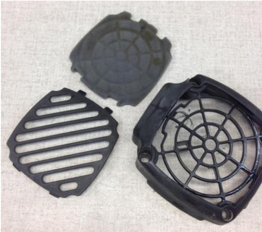
15. Inspect the cap, grill and foam filter for damage. If the foam filter has holes, replace it (P/N: B0095) The foam filter may also be cleaned with soap and water and reused. Allow to dry before reassembly.
