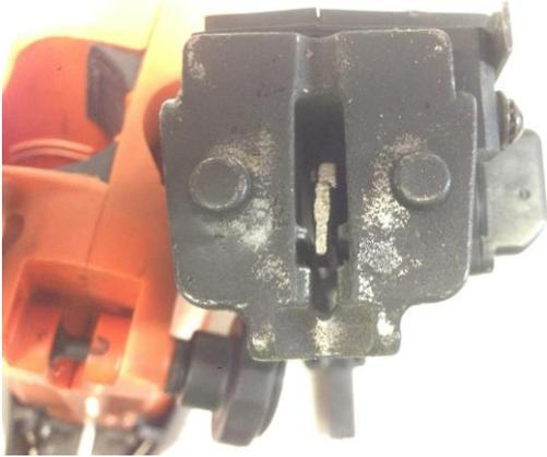
13. On magazine equipped tools, inspect the shear block end of the magazine for debris or damage. Use compressed air to blow out the magazine rails and/or wipe the magazine clean of debris.
