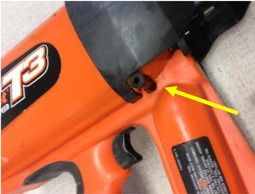
17. Insert the handle bushing into the hex area. See arrow. On the back side of the picture shown insert the screw into the handle bushing and tighten.
