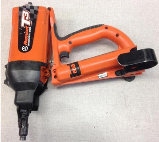
16. The tool can now be reassembled. Place the cylinder head from the handle half assembly into the top of the motor assembly. The hinge point of the cylinder head will allow the handle to be angled as to allow the fuel connector to fit into the side of the housing. Care must be used to not bend the fan blade.
