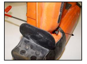
3. After the screw is completely removed, push the Handle/Housing Bushing through the handle
