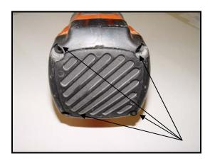
Begin disassembly by removing the four (4) Cap Screws. A 5/32-inch hex key wrench is required for removal.
