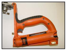
The Handle and Housing assemblies are now separated. Work can now be performed on the assembly needing service.
