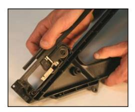
Remove Lockout Bracket screw (part #801122).
