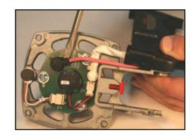
Unplug Spark Wires from Spark Unit.
