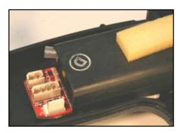
Disconnect Head Switch from P.C. Board (part #404601) and unscrew Head Switch.
