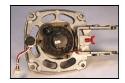
The Motor Sleeve orientation will determine how well the spacing will be around the shaft. Make sure that it is equally spaced all the way around.
