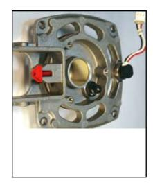
Notice the difference between one end of the Sleeve to the other. One side of the sleeve has a rib. The other side does not. The ribs should be to the inside and should touch the fan motor.
