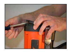
Loosen four screws using a 5/32" hex key (Part # 7405061).
