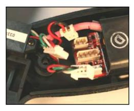
Lift up with screw driver to remove Spark Unit (part #7405163).
