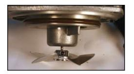
Carefully place the Fan Blade until it is flat and leveled over the Fan Blade Spacer.
