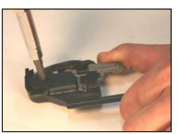
Remove Lockout Bracket (part #801106).
