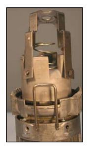
Lift out Mid-check Retaining Ring (part #401322).
